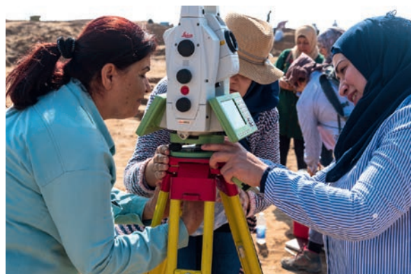
Iraqi archaeologists learning to set up and use a Leica Multi-station, which can be used for point recording and 3D scanning.
